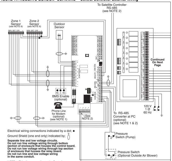
NOTE 1: This diagram applies to the Central Controller (controller #1) only. For all Satellite Controllers see Satellite Controller External Wiring Diagram. Central Controller (controller #1) requires outdoor sensor wiring and either modem, RS-485 converter wiring, or TCP/IP module wiring.
